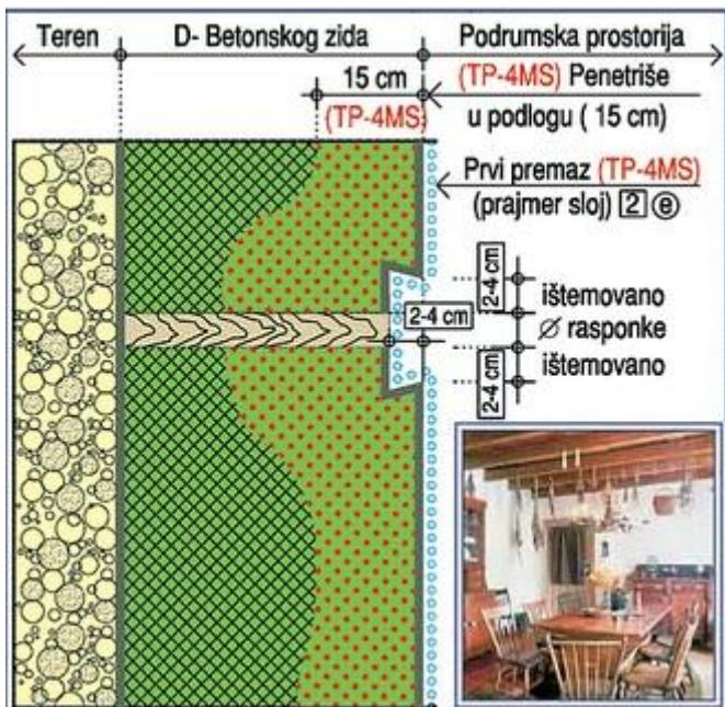
**DETALJ 2e: IZRADA PRVOG PREMAZA TP - 4MS (PRAJMER SLOJA) NA IŠTEMOVANOM ŠLICU KOD RASPONKE (DRVENE, PLASTIČNE I METALNE). ISTO VAŽI I ZA ARMATURU ILI ŽICU KOJA PRODIRE KROZ BETON.**
